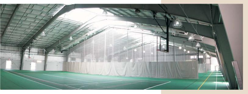
Operable mesh curtains provide protection for those using the track while other sports are taking place, and they also act as dividers between the courts allowing maximum flexibility in the usage of the field house. Orcutt Associates incorporated natural light into the space by means of a skylight running along the ridge of the building and the use of Kalwall translucent panels in the walls.
